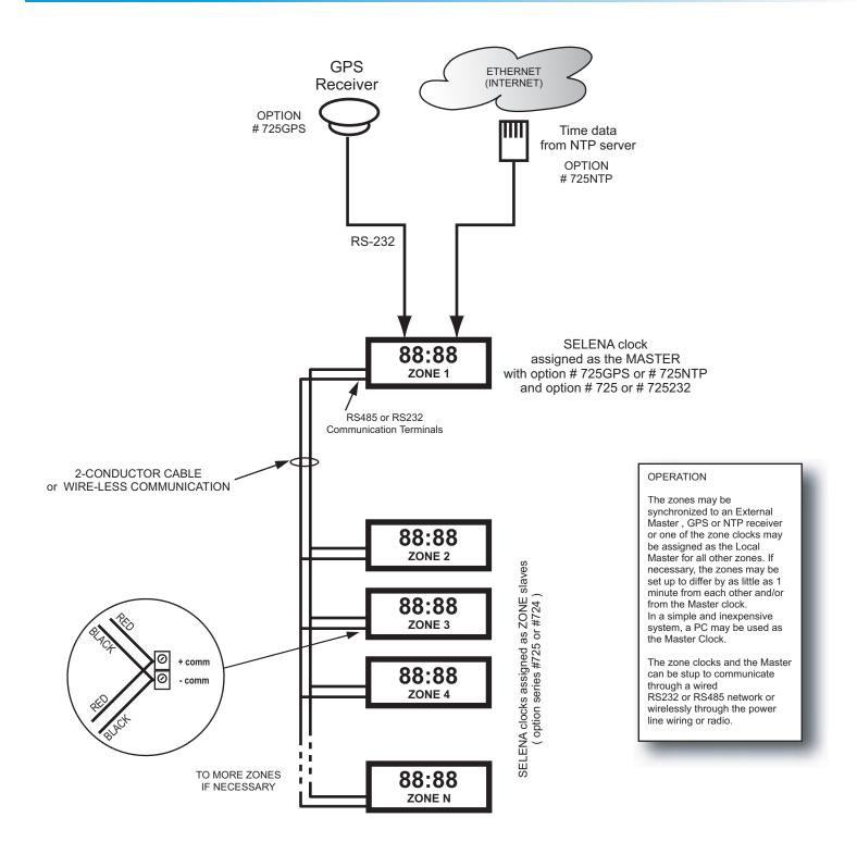
EXAMPLE OF MULTI-ZONE SYSTEM WITH GPS or NTP ATOMIC TIME WITH ZONE CLOCKS HOUSED IN SEPARATE ENCLOSURES
