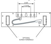
Short cord with flat plug shownOptional:1) Long cord or Screw terminalfor power connection2) Wall plug-in transformer for power
